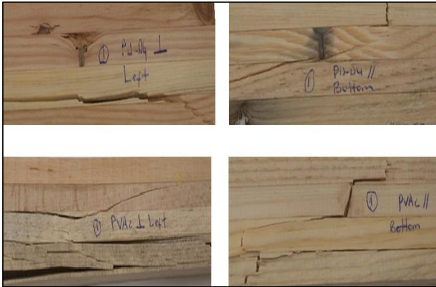
Figure 7: Fracture Types for Bending Test to Perpendicular to The Glue Line and Parallel to The Glue Line
