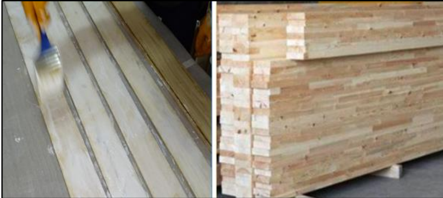
Figure 4: The Glue Solution Was Applied To The Solid Bonding Surfaces With A Brush.
