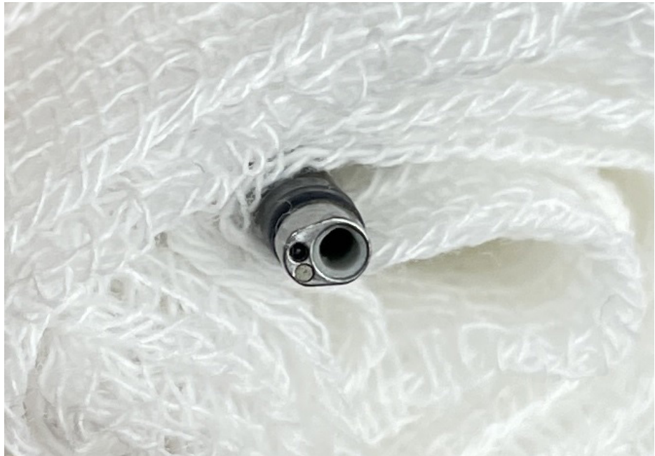
Figure 1/a: Flexible ureteroscope, 1/b: Head of fURS, 1/c: Tip of fURS(Channels of light, water and guideline or laser)
