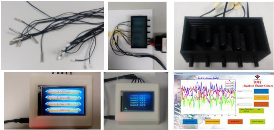
Figure 7. A picture of the UME MEDMET temperature measurement system and NTC-Type thermocouple used in this system
