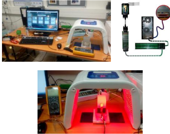
Figure 5. The temperature measurement system and its components for the LED experiment.
