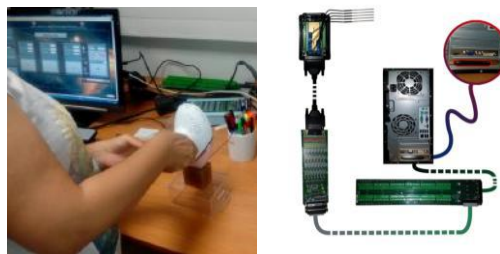
Figure 4. The PC-based temperature measurement system used for the IPL phantom experiment.
