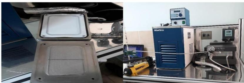
Figure 2: Cross Flow Membrane Filtration System
