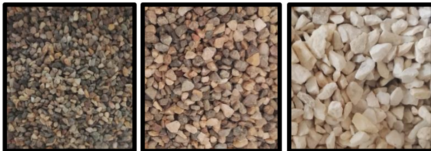
Figure 1. Pervious polymer concrete aggregates
