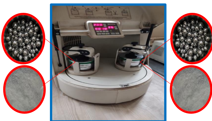
Figure 8. Powders, balls and planetary ball mill used in alloying
