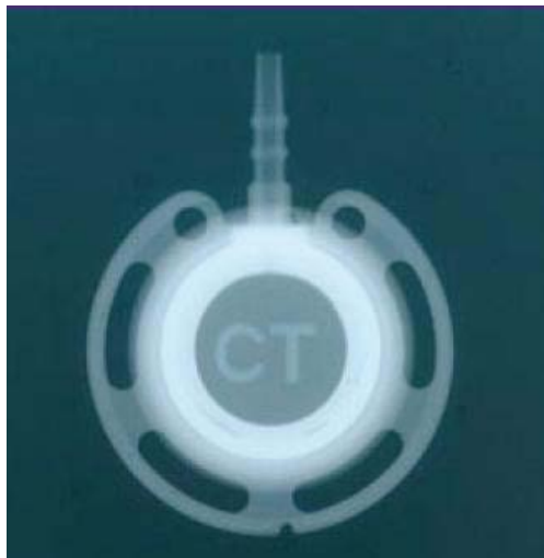
Figure 8.11: Direct radiography of the subcutaneous port produced for high pressure use.
