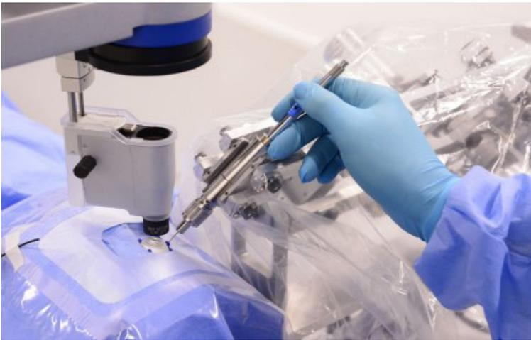
**Figure 2.** The intraocular robotic system of the Catholic University of Leuven. Gijbels A, Smits J, Schoevaerdt L, et al. In-human robot-assisted retinal vein cannulation, a world first. *Ann Biomed Eng.* 2018;46:1676-1685.
