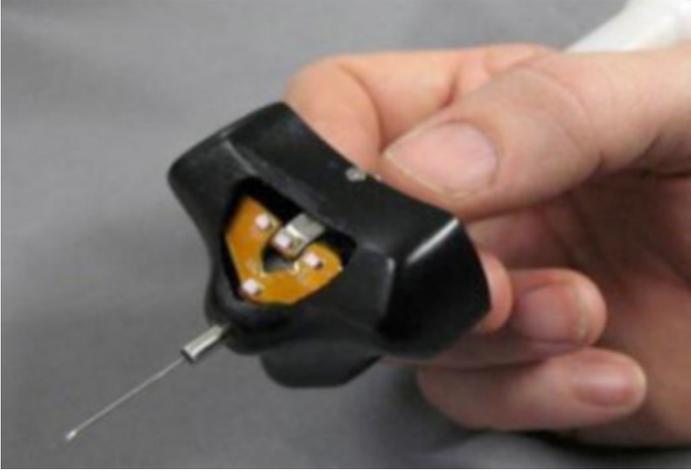
**Figure 1.** The MICRON. A hand-held robotic manipulator.
