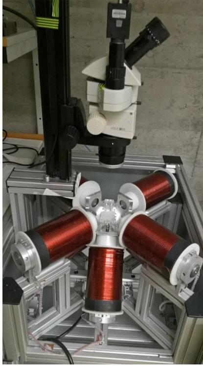
**Figure 9.** Magnetically guided robots, OctoMag. Ahronovich EZ, Simaan N, Joos KM. A review of robotic and OCT-aided systems for vitreoretinal surgery. *Adv Ther.* 2021;38:2114-29.
