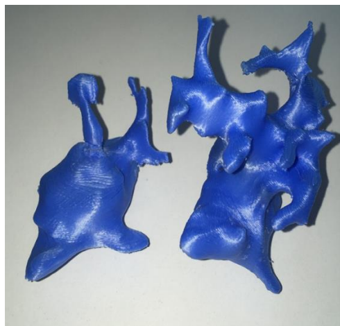
Figure 4: The volumetric change of the mass in one year is presented visually. Solid patterns of the mass from both tomography images were saved in STL format, and the solid models were created with a three-dimensional laser printer using Fused Deposition melting technology with polylactic acid.
