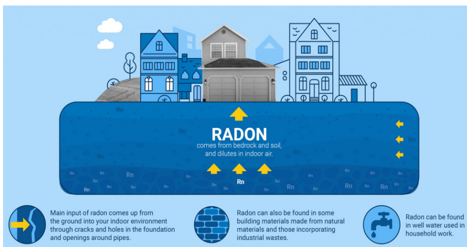
Figure 3. Ways of radon entry into buildings (Adapted from Ref. UNEP 2016; Open-source content for public information)
