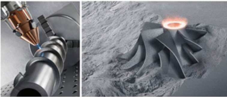
Figure 20. Spiral Part Produced in Additive Manufacturing Machine (Altuncu, 2020)
