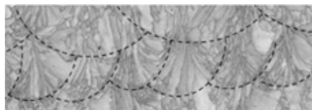
Figure 16. Sectional image for stainless steel fabricated with lmd in 3 layers (Haghdadi et al., 2021)
