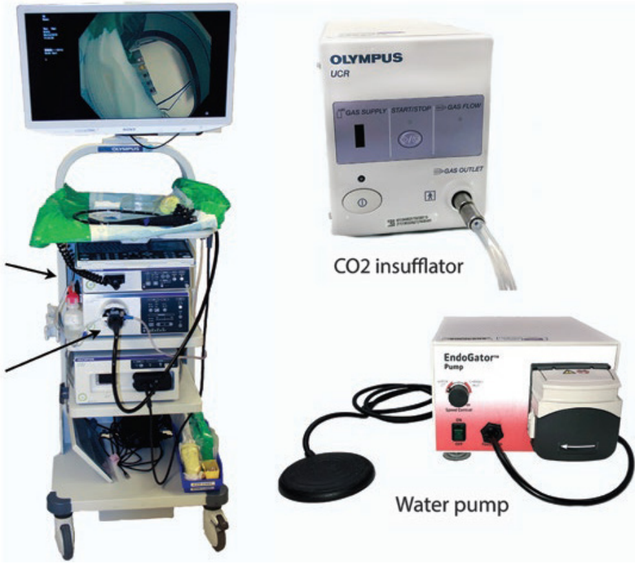
Figure-9: A travel endoscopy tower including components of an image processor (short arrow) and light source (long arrow) (Olympus, Tokyo, Japan). Other frequently used components include a CO2 insufflator (Olympus, Tokyo, Japan), water pump (Medivators, Minneapolis, MN, USA), as well as an energy source
